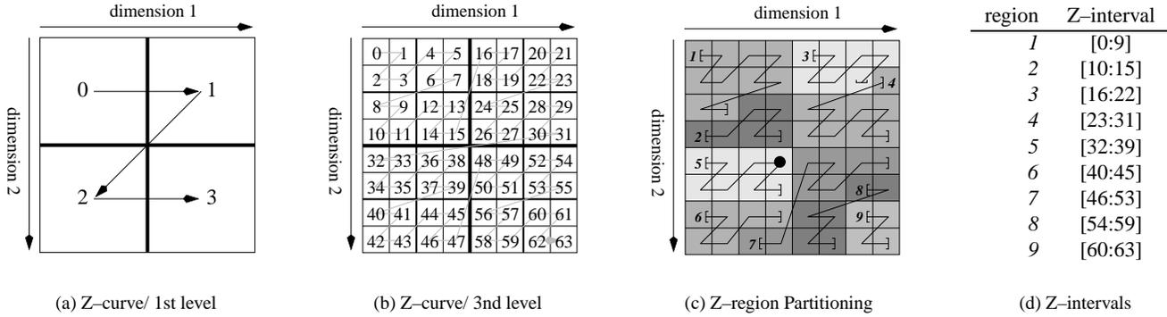
Figure 1. Z-curve and Z-regions used by the UB-Tree
