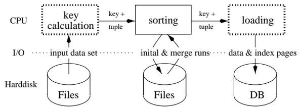
Figure 2. Bulk Loading Architecture for one dimensional clustering indexes
